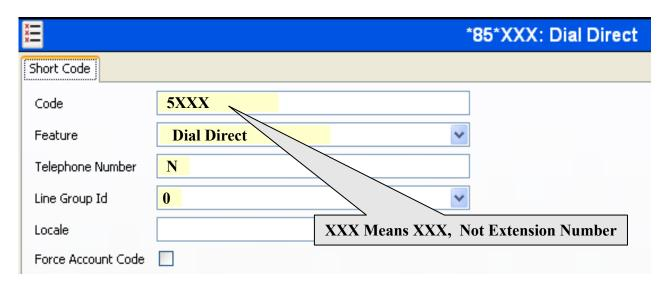
Note: The three X's mean that the IP Office is using 3 Digit Extension Numbers.
